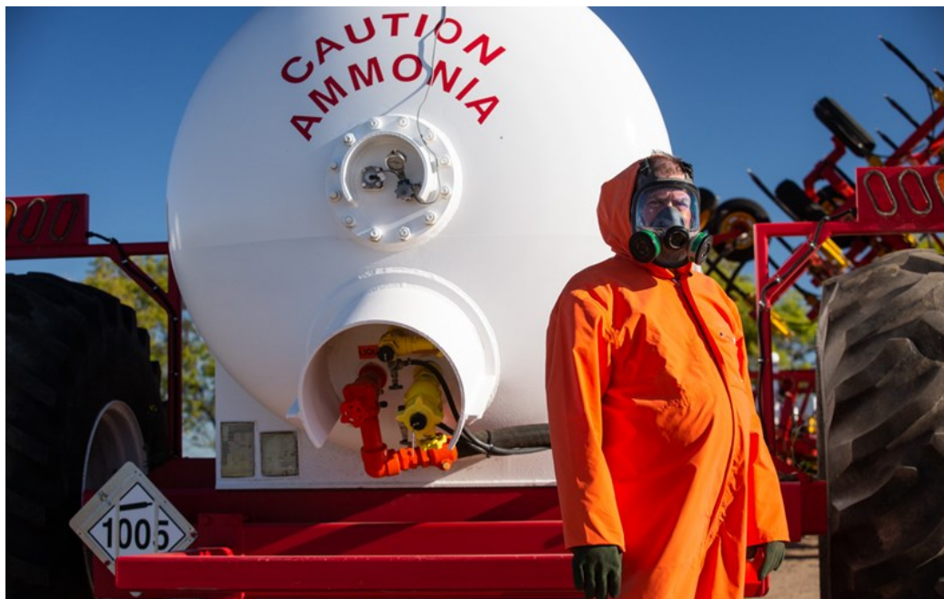
Figure 16. Specialized equipment is required when handling ammonia (credit: fertilizercanada.ca)
