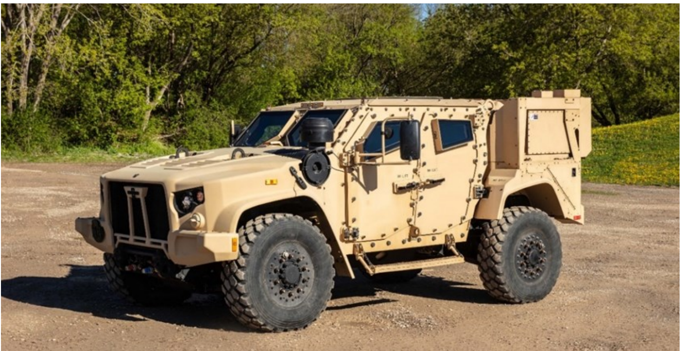
Figure 1. A hybrid electric version of the Joint Light Tactical Vehicle by Oshkosh Defense (credit: oshkoshdefense.com)
