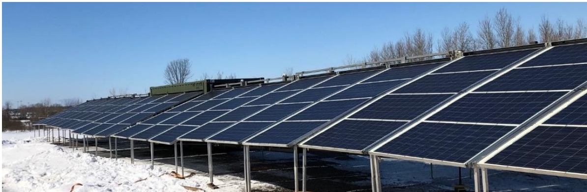
Figure 1. NATO ENSEC COE HPGS Array of PV panels "climate trials" in Canada March 2019. 12
