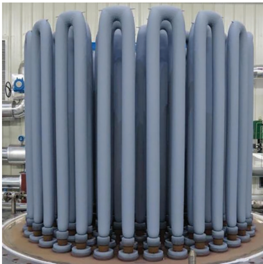
Figure 5. Polysilicon rods grown in a CVD reactor. In this photo the CVD process is complete, the "bell jar" reactor dome has been removed, and the rods are ready for harvest.
