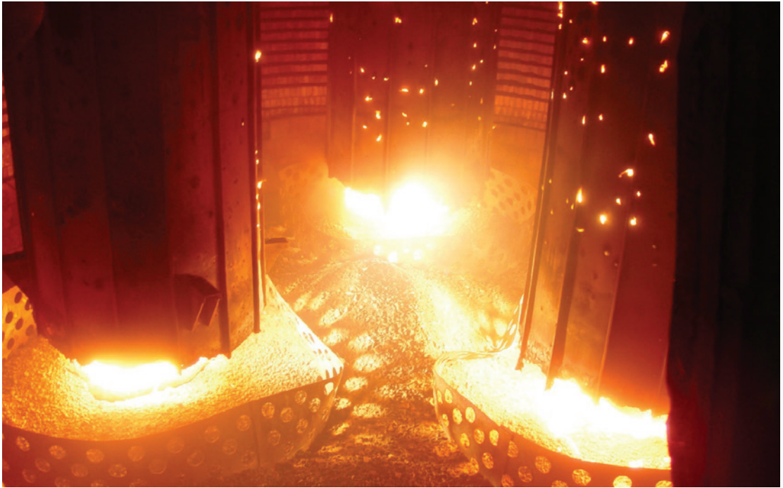
Figure 2. In the silicon smelter, three 1-meter diameter carbon electrodes penetrate the surface of the charge of coal, coke, woodchips, and quartz rock. Each electrode is 10-20 meters tall.
