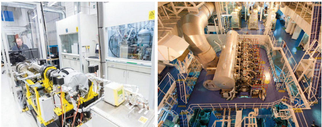
Figure 4: A) Test engine for using NH 3 as fuel in an internal combustion engine in a laboratory at the Wärtsilä Helsinki Campus of the Wärtsilä Corporation (Finland) (Wärtsilä Helsinki Campus 2020). B) Engine test room at MAN Energy Solutions (The Maritime Executive 2020)
