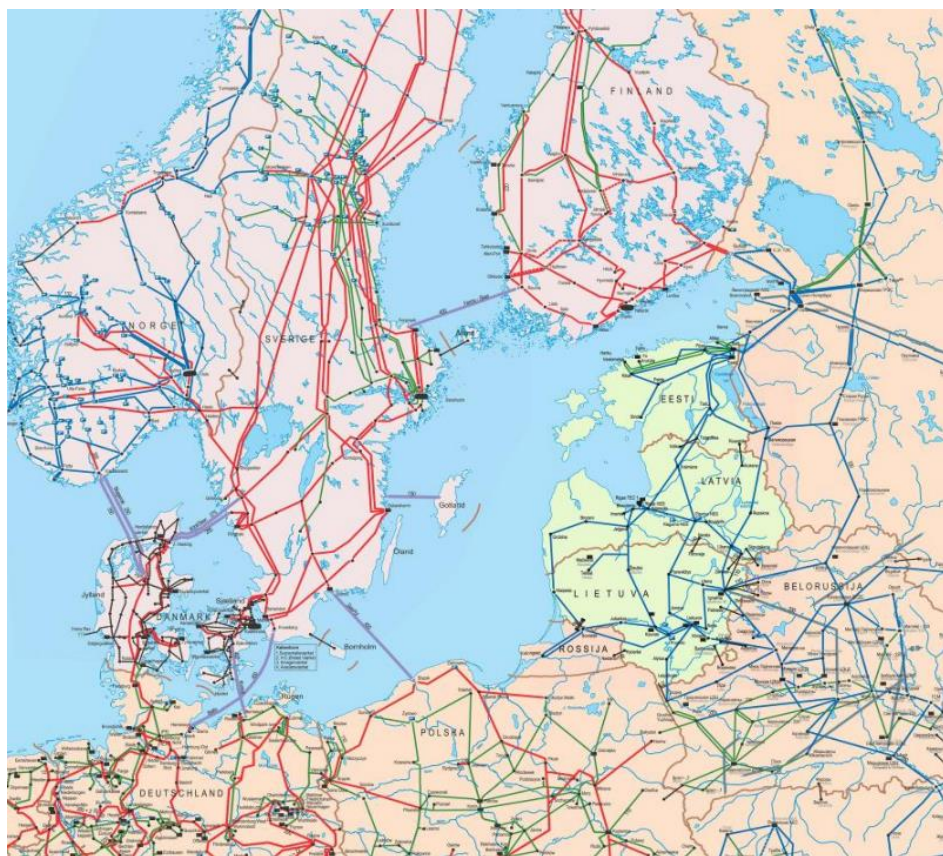
3 Figure. The transmission networks of the Baltic States and Kaliningrad. Source. Energy Analysis. 80
