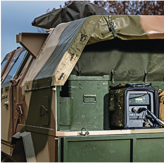
Figure 25: Fuel Cells mounted on German Dingo heavily armored military MRAP
