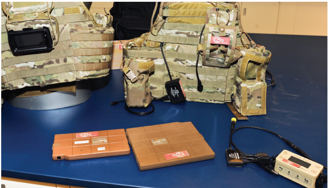
Figure 13: Conformal Wearable Batteries
