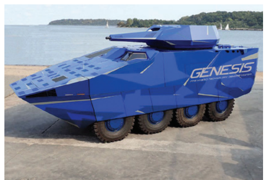
Figure 23: GENESIS 8x8 - full hybrid technology demonstrator, based on BOXER multirole armoured fighting vehicle
