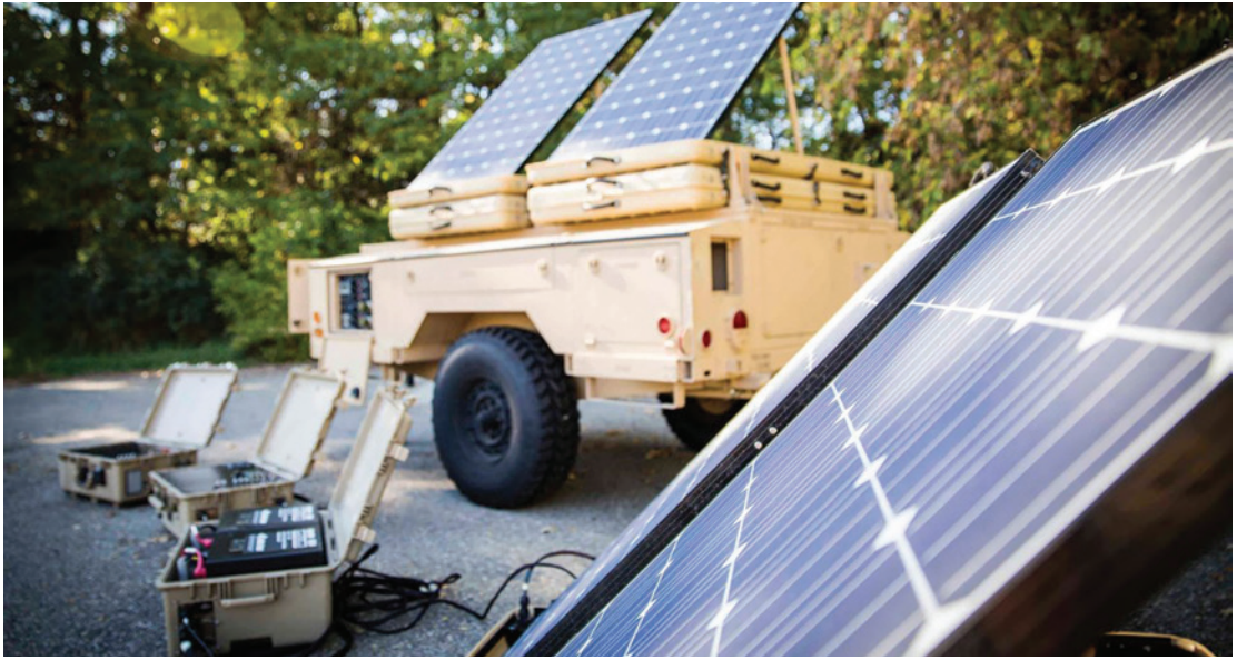
Figure 14: Tactical Mobile Microgrid System
