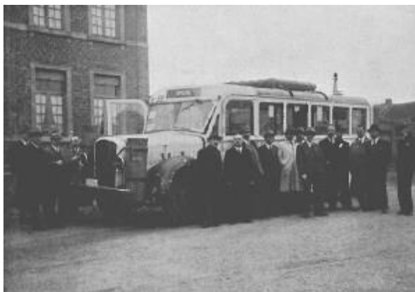
Figure 1: Retrofitted bus with an ammonia driven internal combustion engine in 1943 during WWII in Belgium (Kroch 1945).
