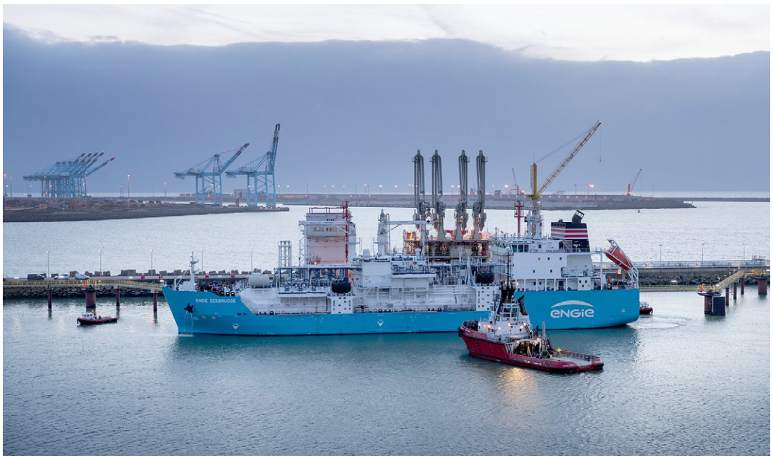
Figure 13 – The bunkering vessel ENGIE Zeebrugge is jointly owned by ENGIE, Mitsubishi Corporation, NYK Line, and Fluxys. With an LNG capacity of 5,000 m 3 , she will service all types of shipping customers in Northern Europe from her home port of Zeebrugge, under the brand Gas4Sea
