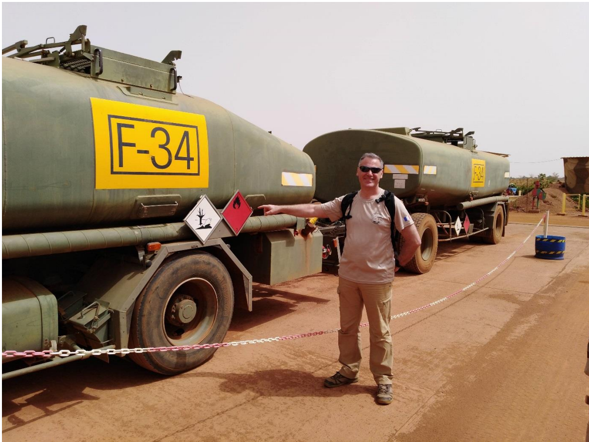
Figure 1: Fuel truck of the French Army Corps d' Essence in a field camp in Niger loaded with NATO F-34 fuel. The fossil carbon based F-34 is currently the standard liquid fuel for military aviation and also the basis of truck diesel in NATO forces. 45
