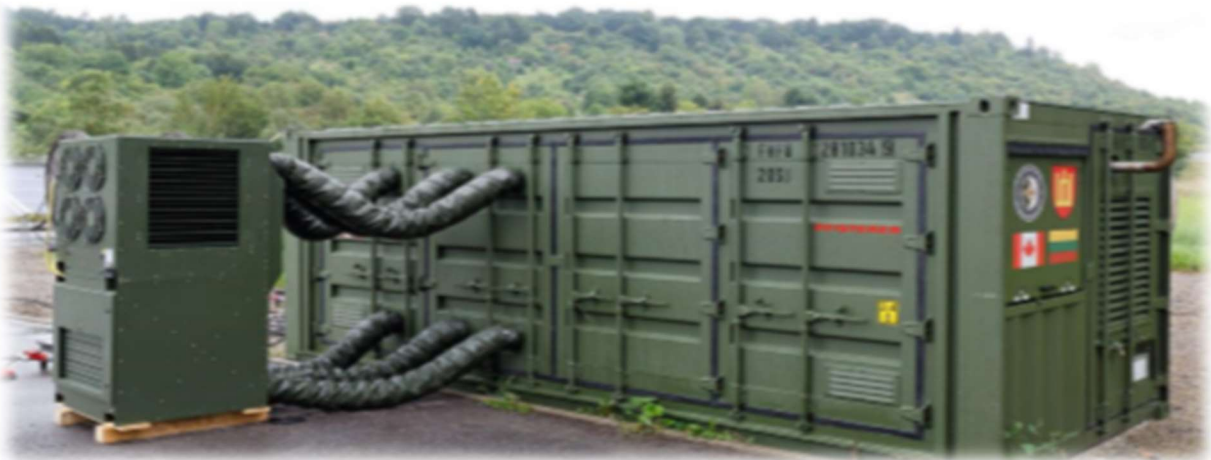
Figure 23. External heating/cooling unit (Pfisterer, 2017)
