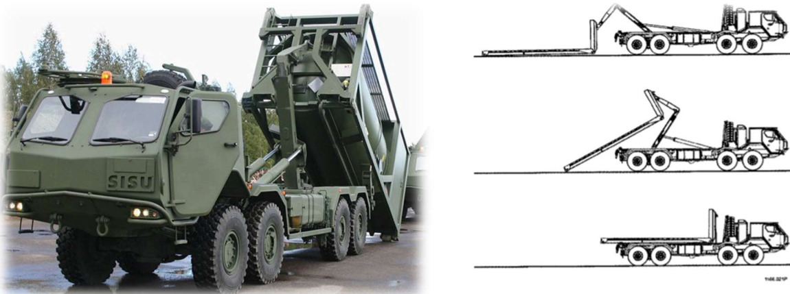
Figure 24a. SISU E13 TP8x8 truck with integrated Multilift model MHS135 during loading Figure 24b. SISU loading diagram (SISU documentation)
