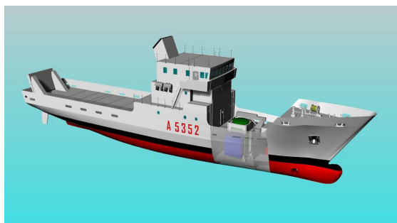
Figure 4. LNG fueling system installation on board of Italian navy's Ro-Ro vessel.
